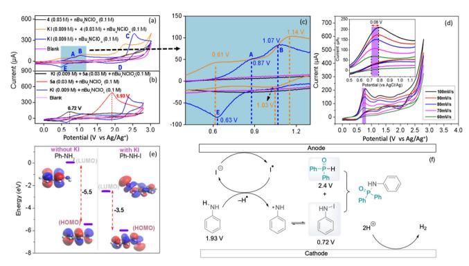
Fig. 5 Mechanistic investigation with cyclic voltammetry: (a) CV of 4 and KI, (b) CV of aniline and KI, (c) expansion of plot (a), (d) CV at different scan rates (inset: variation in peak current and shift in potential), (e) HOMO–LUMO energy gap with and without KI, and (f) proposed mechanism.
