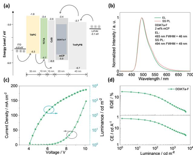
Fig. 5 (a) Device configuration and energy levels for each layer; (b) electroluminescence spectra for devices; (c)  $J$ - $V$ - $L$  characteristics; and (d) EQE and CE versus luminance characteristics.
