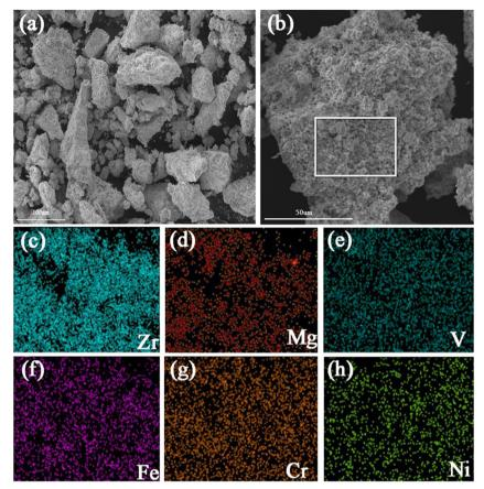
Fig. 3 SEM images (a) and (b) and EDS mappings (c)–(h) of the Zr<sub>2</sub>MgVFeCrNi high-entropy alloys.
