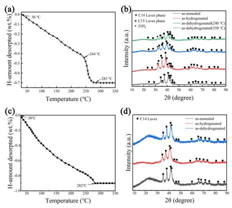
Fig. 7 TPD profile of (a)  $Zr_2MgV_2CrNi$  and (c)  $Zr_2MgVFeCrNi$  high-entropy alloys at a heating rate of 5 °C min<sup>-1</sup>, as well as their XRD patterns for (b) Zr<sub>2</sub>MgV<sub>2</sub>CrNi and (d) Zr<sub>2</sub>MgVFeCrNi high-entropy alloys at different states
