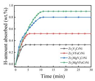
Fig. 5 Hydrogen absorption kinetics curves of  $Zr_2Mg_xV_{2-y}Fe_yCrNi$  (x = 0 and 1, and y = 0 and 1) high-entropy alloys at 303 K.
