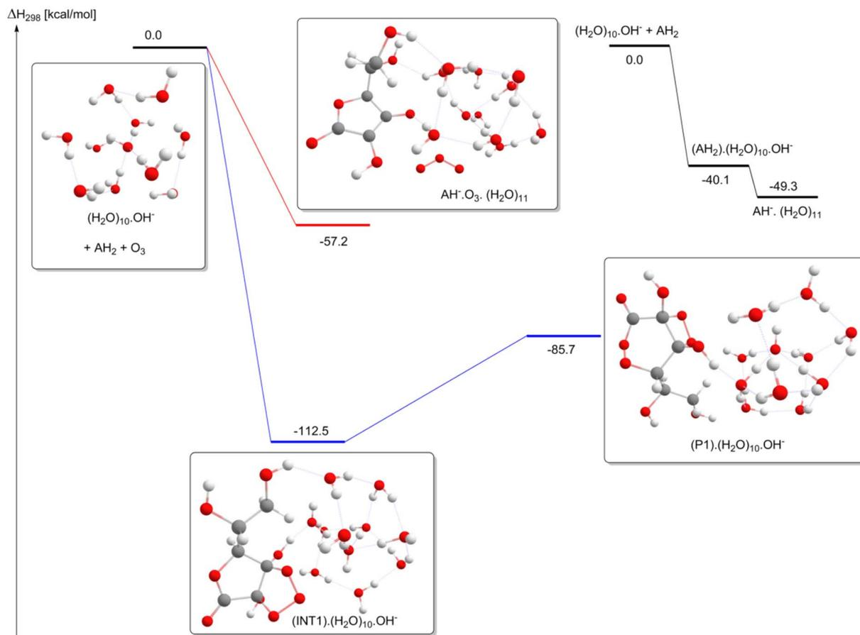
Fig. 8 Enthalpies ( $\Delta H_{298}$ , kcal mol<sup>-1</sup>) calculated for the reactions between ascorbic acid and O<sub>3</sub> on the [(H<sub>2</sub>O)<sub>10</sub>·OH<sup>-</sup>] surface.
