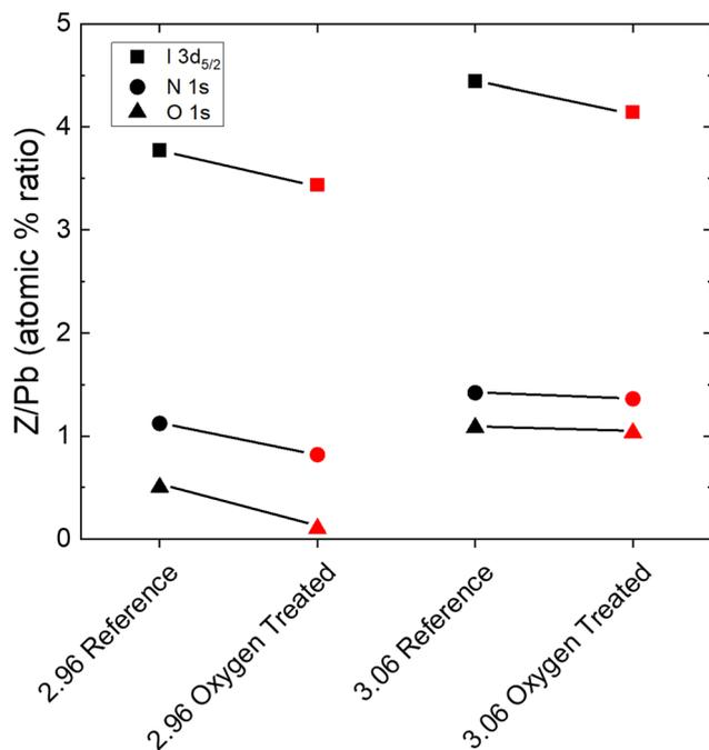
Fig. 4 The atomic percentage ratios of iodine, nitrogen, and oxygen relative to the Pb4f<sub>7/2</sub> doublet for an understoichiometric and overstoichiometric sample. All ratios decrease upon photooxygen treatment.
