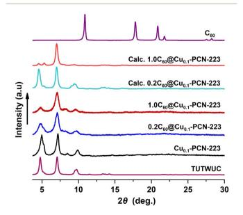
Fig. 2 PXRD data for  $Cu_{0.1}$ -PCN-223 and the  $C_{60}$ @ $Cu_{0.1}$ -PCN-223 composites vs. PXRD data for PCN-223 simulated from the single crystal diffraction data (Cambridge Crystallographic Data Centre (CCDC) code: TUTWUC) and two fulleretic composites optimized in this study (please see Section 2.2).
