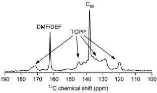
Fig. 4 (Up) <sup>1</sup>H MAS NMR spectra for Cu<sub>0.1</sub>-PCN-223 and  $1.0C_{60}$ @Cu<sub>0.1</sub>-PCN-223 at 300 K. (Down)  $^{13}$ C MAS NMR spectrum of 1.0C<sub>60</sub>@Cu<sub>0.1</sub>-PCN-223 at 300 K. The signals from dimethylformamide (DMF), diethylformamide (DEF), H<sub>2</sub>TCPP linker and fullerene (C<sub>60</sub>) are indicated on the spectra.
