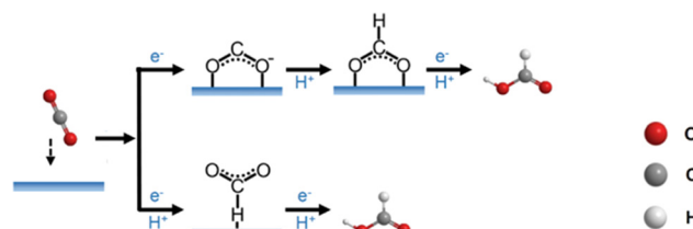
Fig. 7 Schematic diagram of the 2\text{e}^- reaction path in \text{eCO}_2\text{RR} . Copyright 2021, Elsevier. 65
