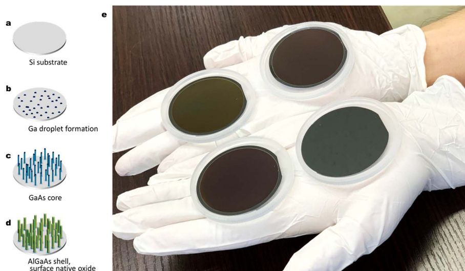
Fig. 1 (a)–(d) Procedure for the formation of nanowires on a Si substrate. (e) 2-Inch Si wafers before (front right) and after (others) nanowire growth. Samples after nanowire growth show a dark-colored feature indicating light absorption on the substrate surface, except for the periphery where the substrate was held during growth. The slightly different colors of the nanowire samples reflect the slight difference in the Al composition and thickness of the outermost AlGaO x shells for each nanowire sample.
