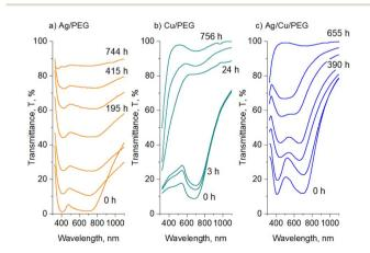
Fig. 5 Time evolution of the UV-vis transmittance spectra of: (a) Ag/ PEG, (b) Cu/PEG, and (c) Ag/Cu/PEG nanofluids. The NP mean size is 30 nm, the total metal concentration is 50  $\mu$ g mL<sup>-1</sup> (25  $\mu$ g mL<sup>-1</sup> Ag and 25  $\mu$ g mL<sup>-1</sup> Cu, in the case of Ag/Cu/PEG).
