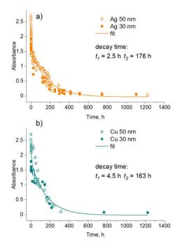
Fig. 8 Attenuation of LSPR absorbance maxima with time for NPs of 30 and 50 nm mean sizes during their sedimentation: (a) Ag; (b) Cu. The total metal concentration is 50  $\mu g$  mL<sup>-1</sup>. The lines are fit by a two-exponential decay.
