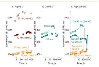
Fig. 7 Change in the LSPR position with time for nanofluids with NPs of mean sizes of 30 and 50 nm: (a) Ag/PEG, (b) Cu/PEG, and (c) Ag/Cu/PEG. The total metal concentration is 50  $\mu g\ mL^{-1}$  (25  $\mu g\ mL^{-1}$  Ag and 25  $\mu g\ mL^{-1}$  Cu, in the case of Ag/Cu/PEG). Data points placed on the y-axes belong to time =0 h.
