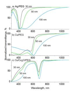
Fig. 6 Simulated UV-vis transmittance spectra of: (a) Ag/PEG, (b) Cu/ PEG, and (c) Cu/Cu<sub>2</sub>O/PEG nanofluids with NPs of different mean sizes. The NPs are distributed lognormally with a standard deviation of 20%. For the core/shell Cu/Cu<sub>2</sub>O NPs, the radius of the Cu core is egual to the thickness of the Cu<sub>2</sub>O shell. The spectra are normalized in the range 0 to 100%.
