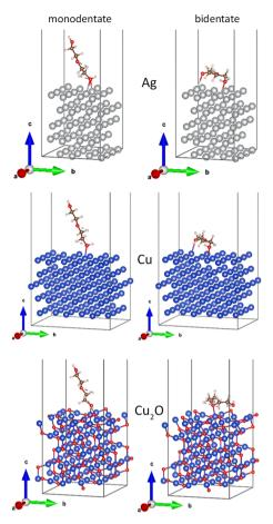
Fig. 12 Relaxed interface geometries of DEG onto the Ag(111), Cu(111), and Cu<sub>2</sub>O(111) surfaces. Left column: monodentate configuration and the right column: bidentate configuration.
