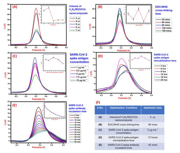
Fig. 5 The optimization data for the fabrication of the immunosensor; (A) volume of C<sub>3</sub>N<sub>4</sub>/RGO/Chi nanocomposite, (B) EDC/NHS cross-linker incubation time, (C) SARS-CoV-2 spike antigen concentration, (D) SARS-CoV-2 spike antigen immobilization time, and (E) SARS-CoV-2 antibody incubation time, 0.1 M PBS (pH 7.4) containing 0.1M KCl and 5 mM ferri/ferrocyanide redox solution, (F) the summarized optimization data in tabular format.
