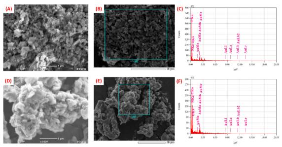
Fig. 3 SEM images of (A) and (B)  $C_3N_4/RGO$  and (D) and (E) bio-functionalized  $C_3N_4/RGO$  nanocomposite. Elemental distribution of (C)  $C_3N_4/RGO$  and (F) bio-functionalized C<sub>3</sub>N<sub>4</sub>/RGO nanocomposite respectively.
