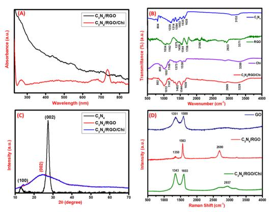
Fig. 1 (A) UV-vis spectra of  $C_3N_4/RGO$ , and  $C_3N_4/RGO/Chi$  nanocomposite (B) FTIR spectra of  $C_3N_4$ , RGO, Chi, and  $C_3N_4/RGO/Chi$  nanocomposite, (C) XRD patterns of  $C_3N_4$ ,  $C_3N_4$ /RGO, and  $C_3N_4$ /RGO/Chi nanocomposite, and (D) Raman spectra of GO,  $C_3N_4$ /RGO, and  $C_3N_4$ /RGO/Chi nanocomposite.
