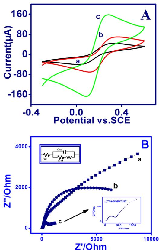
**Fig. 2** (A) Cyclic voltammetry and (B) electrochemical impedance spectra on PIGE (curve *a*), MWCNT (curve *b*) and TSAB/MWCNT (curve *c*) in 1 mM [Fe(CN)<sub>6</sub>]<sup>-3/4-</sup> containing 0.1 mol L<sup>-1</sup> ABS (pH-5.0) at 50 mV s<sup>-1</sup>. Inset: Enlarged image of (B) depicting the EIS of TSAB/MWCNT-modified electrode.
