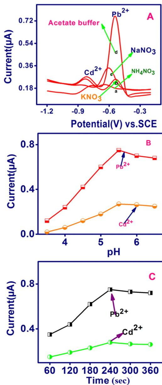
Fig. 4 Effect of (A) supporting electrolyte, (B) pH and (C) preconcentration time on the anodic stripping peak currents of  $\text{Pb}^{2+}$  and  $\text{Cd}^{2+}$  (8 ppb each) to evaluate TSAB/MWCNT sensor performance in 0.1 M ABS (pH 5.5).
