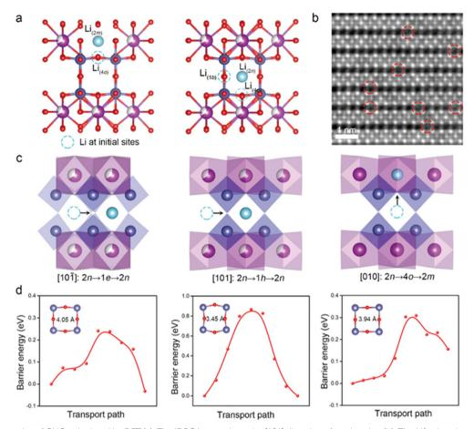
Fig. 7 Li<sup>+</sup> insertion point of CNO calculated by DFT (a). The iDPC image along the [101] direction after charging (b). The Li<sup>+</sup> migration pathway (c) and the energy profile (d).87 Copyright © 2022 Wiley VCH.
