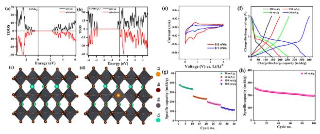
Fig. 2 TDOS of CsPbBr<sub>3</sub> without (a) and with Li<sup>+</sup> (b). Side views (c and d). CV curves (e), GCD curves (f), specific discharge capacity (g), and cycling diagram (h) of CsPbBr<sub>3</sub>. 48 Copyright © 2021 American Chemical Society.
