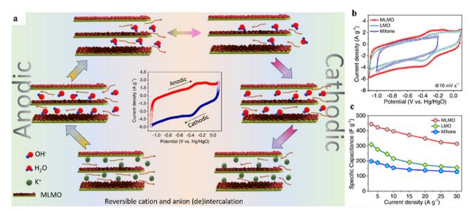
Fig. 14 Schematic illustration of reversible cation and anion (de)intercalation in MLMO (a). Comparison of CV curves (b) and specific capacitances (c) of LMO, MXene and MLMO. 152 Copyright © 2022 Elsevier.
