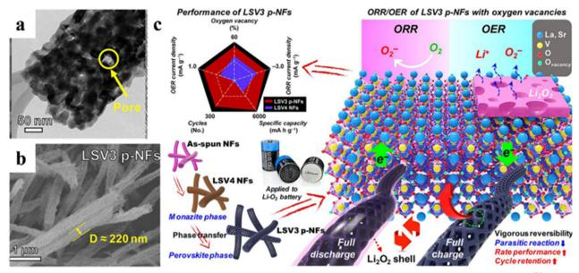
Fig. 13 TEM (a) and SEM (b) of La<sub>0.8</sub>Sr<sub>0.2</sub>VO<sub>3</sub> (LSV3 p-NFs). Schematic illustration of LSV3 p-NFs used in rechargeable Li-O<sub>2</sub> batteries (c). <sup>136</sup> Copyright © 2020 Elsevier.
