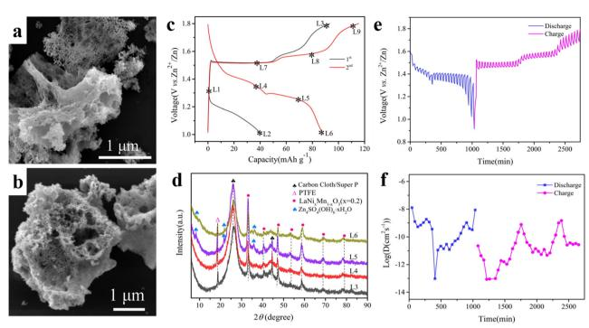
Fig. 11 SEM of LaNi<sub>x</sub>Mn<sub>1-x</sub>O<sub>3</sub> (x = 0.2) (a) and LaMnO<sub>3</sub> (b). Charge/discharge curves (c), XRD at different voltages (d), GITT curves (e) and diffusion coefficients (f) of LaNi<sub>x</sub>Mn<sub>1-x</sub>O<sub>3</sub> (x = 0.2). Copyright © 2022 Elsevier.
