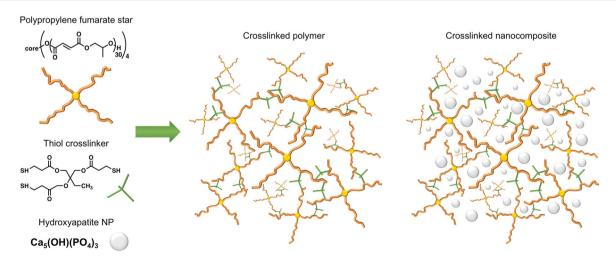
Fig. 1 Poly(propylene fumarate) 4-arm star polymers were crosslinked photochemically using a Carbon M2 printer and a crosslinker with three pendent thiol groups. Hydroxyapatite nanopowder was added to the resin and printed to yield nanocomposites. Tensile bars, DMA bars, and gyroid scaffolds were 3D printed and subjected to different post-curing conditions.
