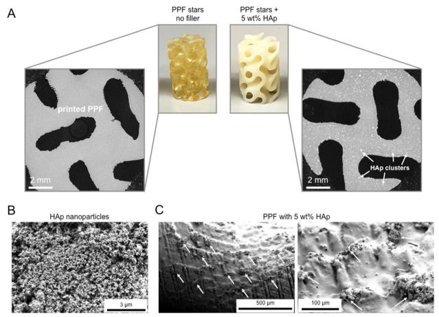
Fig. 2 Each of the printed scaffold materials was evaluated by μCT and SEM in order to observe the microstructure. (A) μCT measurements confirmed the presence of HAp clusters post-printing compared to the pure PPF. (B) HAp nanoparticles were observed with SEM to be uniform. (C) Individual HAp nanoparticles and aggregates were observed on the surface of the printed structures.
