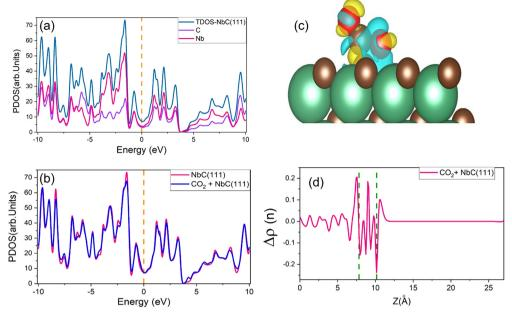
Fig. 4 (a) The PDOS for the NbC (111) surface, (b) the TDOS of NbC (111) prior to and after adsorption of CO2, (c) view of the charge density differences, with the C and O atoms illustrated in brown and red (isovalue =  $\pm 0.002$ ) and, (d) the planar average charge density. The Fermi level is set at zero.
