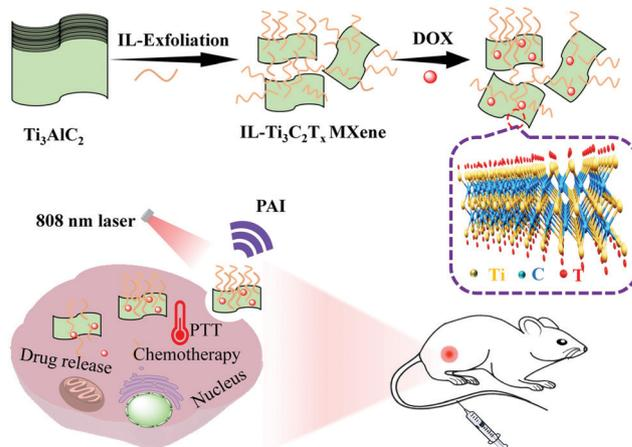
**Scheme 1** Schematic illustration of the preparation of few-layer  $\text{Ti}_3\text{C}_2\text{T}_x$  MXene nanosheets with high chemical stability using an IL-assist exfoliating method. The nanosheets can be used for photoacoustic imaging and the synergistic photothermal/chemotherapy of tumors.
