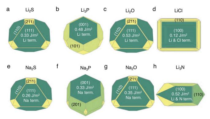
Fig. 1 Computed Wulff shapes of binary compounds  $Li_2S$  (panel a),  $Li_3P$  (b),  $Li_2O$  (c), LiCl (d),  $Na_2S$  (e),  $Na_3P$  (f),  $Na_2O$  (g), and  $Li_3N$  (h), with their corresponding surface energies (in J m<sup>-2</sup>). The chemical nature of the surface terminations (term.) are also indicated. Wulff polygons are constructed using stoichiometric, non-polar, and symmetric surfaces (including an inversion symmetry).
