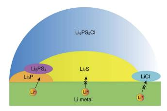
Fig. 5 Schematic illustration of a possible structure of the interface between Li metal and argyrodite-Li<sub>6</sub>PS<sub>5</sub>Cl, as inferred from the interfacial energetics and Li-ion transport simulations.
