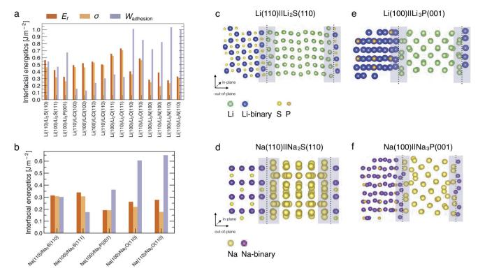
Fig. 2 Computed interfacial quantities (in J m<sup>-2</sup>) for (a) Li-based interfaces and (b) Na-based interfaces. Atomic structures of representative interfaces, namely (c) Li(110)  $\|\text{Li}_2\text{S}(110)$ , (d) Na(110)  $\|\text{Na}_2\text{S}(110)$  (e) Li(100)  $\|\text{Li}_3\text{P}(001)$  and (f) Na(100)  $\|\text{Na}_3\text{P}(001)$ . The interface regions are indicated by the shaded areas. The non-periodic direction of the interface is indicated by the "out-of-plane" vectors.
