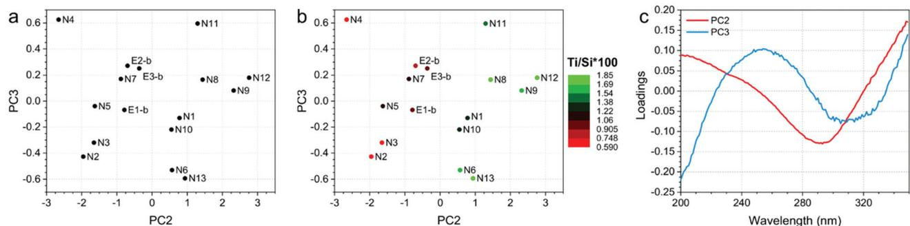
**Fig. 5** (a) PC2 and PC3 scores plot, (b) PC2 and PC3 scores plot, in which the sample spots were scaled according to the  $\text{Ti/Si} \times 100$  and (c) loadings plots of the PCA model developed on DR-UV data.
