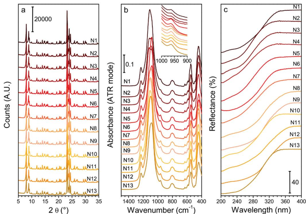
**Fig. 1** (a) XRD patterns of the as synthesized full set of DoE samples; (b) ATR-IR spectra of the activated DoE samples; the inset reports the magnification of  $960 \text{ cm}^{-1}$  signal. (c) DR-UV spectra of the activated DoE samples.
