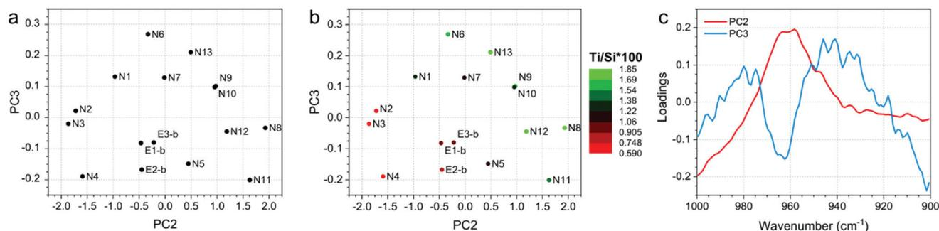
**Fig. 4** (a) PC2 and PC3 scores plot, (b) PC2 and PC3 scores plot, in which the sample spots were scaled according to the  $\text{Ti/Si} \times 100$  and (c) loadings plot of the PCA model developed on ATR-IR data.
