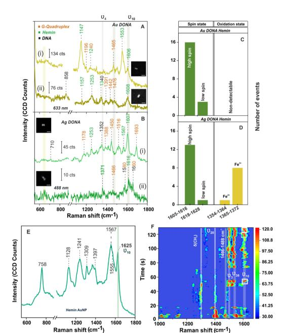
generate Au and Ag DONAs. Fig. 3A(i) shows SM-SERS spectra of the complex unit using Au DONAs (633 nm). A vibrational band attributed to asymmetrical stretching mode ( $C_{\alpha}C_{m}$ ) characteristic of the high spin configuration of hemin appears at 1606 cm<sup>-1</sup> ( $\nu_{10}$ ) along with a sharp band appearing at 1553 cm<sup>-1</sup> ( $B_{1g}$ ) corresponding to  $\nu_{11}(C_{\beta}-C_{\beta})_{asym}$  stretching of
