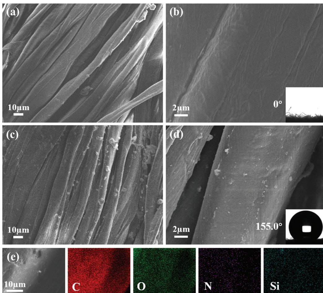
**Fig. 1** SEM photographs of (a and b) the pristine fabric and (c and d) the PEI/TMSPA/SiO<sub>2</sub>/DTMS fabric with 7.5 mg mL<sup>-1</sup> SiO<sub>2</sub> nanoparticles. The insets in (b) and (d) are corresponding WCAs. (e) SEM-EDS mapping image of the coated fabric.
