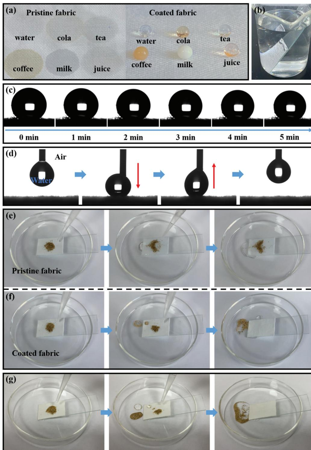
**Fig. 5** (a) Photographs of aqueous droplets on original and coated fabrics. (b) The mirror appearance of the coated fabric that was forcibly put in water. (c) The water droplets staying on the coated fabric show stable superhydrophobicity. (d) Photos of the coated fabric, which repels a 4  $\mu\text{L}$  water droplet. Optical images of self-cleaning tests of (e) pristine and (f) coated fabrics. (g) Self-cleaning performance test of the coated fabric which is contaminated by oil (*n*-hexane).
