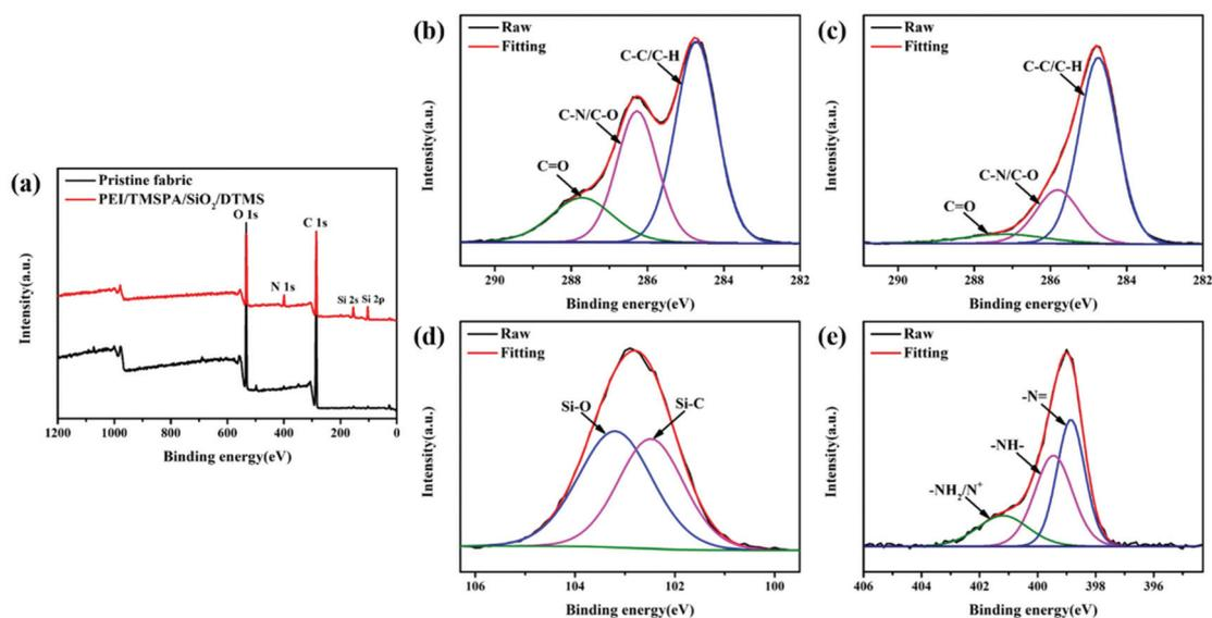
Fig. 3 (a) XPS spectra of pristine and PEI/TMSPA/SiO<sub>2</sub>/DTMS fabrics. C 1s XPS spectra with fitting curves of (b) pristine and (c) PEI/TMSPA/SiO<sub>2</sub>/DTMS fabrics. (d) Si 2p XPS spectra and (e) N 1s XPS spectra with fitting curves of the PEI/TMSPA/SiO<sub>2</sub>/DTMS fabric.
