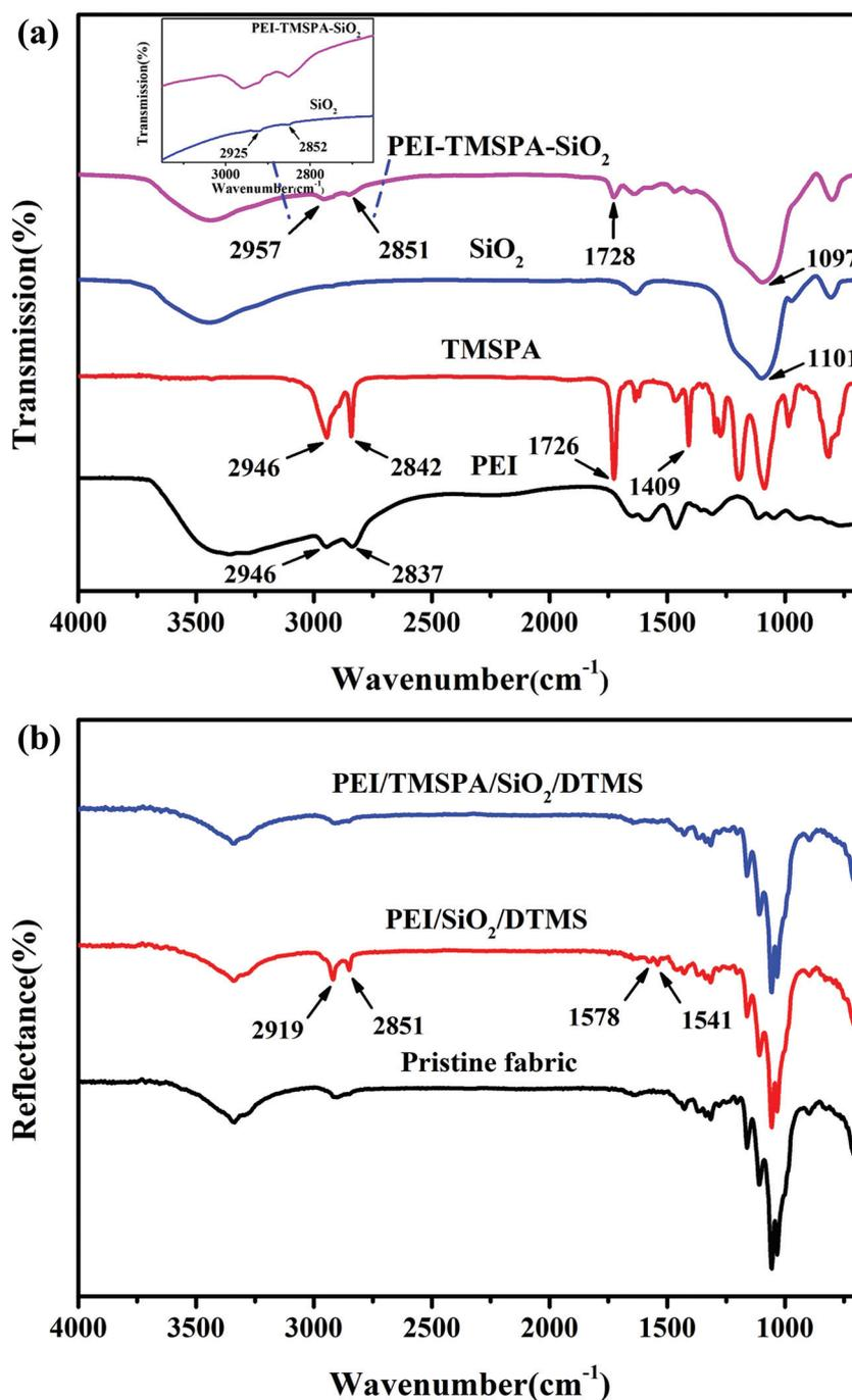
Fig. 2 FTIR spectra of (a) PEI-TMSPA-SiO<sub>2</sub>, pure SiO<sub>2</sub>, TMSPA and PEI, and (b) pristine fabric, PEI/SiO<sub>2</sub>/DTMS fabric and PEI/TMSPA/SiO<sub>2</sub>/DTMS fabric.
