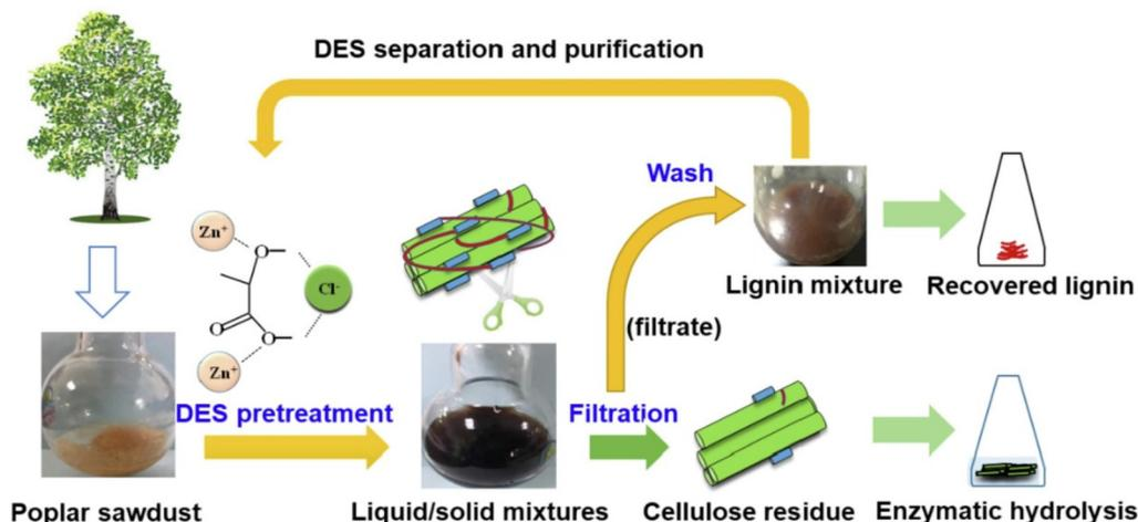
Fig. 2 Schematic representation of the DESs pre-treatment process. Reprinted with permission from ref. 58. Copyright 2022, Elsevier.
