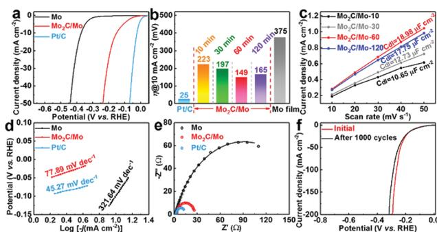
**Fig. 5** (a) Polarization curves of the prepared Mo<sub>2</sub>C/Mo-60, bare Mo plate and Pt/C catalysts at 5 mV s<sup>-1</sup> in 0.5 M H<sub>2</sub>SO<sub>4</sub> at 25 °C. (b) Overpotentials at 10 mA cm<sup>-2</sup>. (c) Linear relationship between the capacitance current density and scan rate. (d) Corresponding Tafel plots and (e) EIS Nyquist plots of different samples. (f) Polarization curves of Mo<sub>2</sub>C/Mo-60 before and after 1000 cycles.
