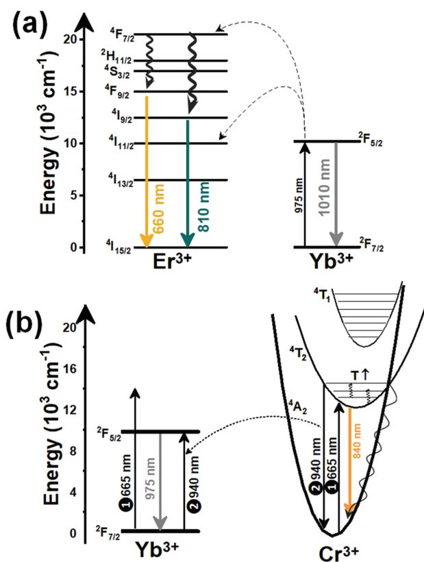
Fig. 24 Mechanisms of generation of the emission lines of dual-doped (a) Er<sup>3+</sup>/Yb<sup>3+</sup> and (b) Cr<sup>3+</sup>/Yb<sup>3+</sup> materials operating simultaneously in the I- and II-BWs.
