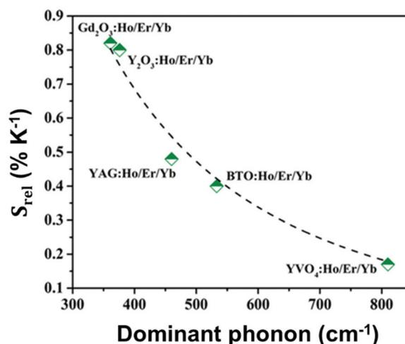
**Fig. 36**  $S_{\text{rel}}$  of  $\text{Er}^{3+}, \text{Ho}^{3+}, \text{Yb}^{3+}$ -co-doped nanoparticles as a function of the dominant phonon energy. Reprinted with permission from ref. 254. Copyright 2020, Wiley-VCH Verlag GmbH & Co. KGaA.
