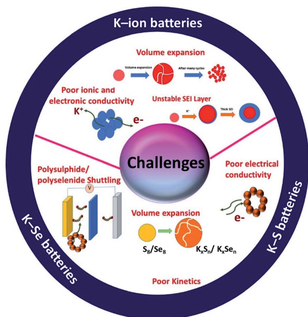
Fig. 3 Schematic of the challenges of potassium batteries.
