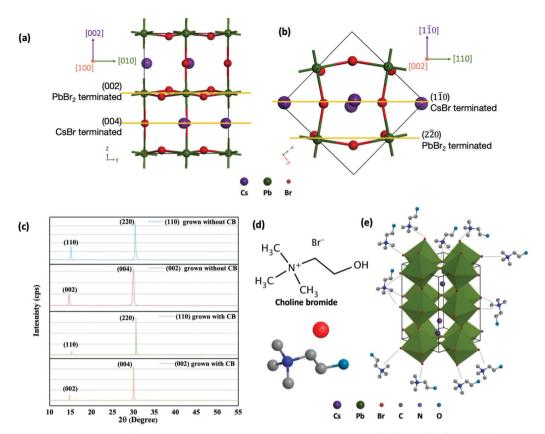
Fig. 2 (a) Side view of the orthorhombic CsPbBr<sub>3</sub> unit cell structure. The yellow lines indicate (002) and (004) plane. (b) Top view of the unit cell structure. The yellow lines indicate  $(1\bar{1}0)$  and  $(2\bar{2}0)$  plane. (c) XRD pattern of CsPbBr<sub>3</sub> single crystal grown with and without CB. (d) Molecular structure of choline bromide (CB). (e) Schematic illustration of CB assisted CsPbBr<sub>3</sub> single crystal growth.
