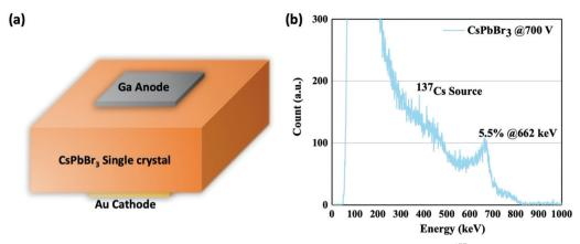
Fig. 4 (a) Schematic of detector structure (4.5 mm × 4.5 mm electrode area, 2.5 mm thickness). (b) 662 keV <sup>137</sup>Cs spectrum acquired by CsPbBr<sub>3</sub> single crystal under 700 V.
