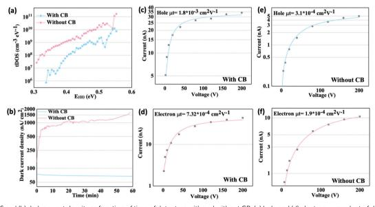
Fig. 3 (a) tDOS and (b) dark current density as function of time of detectors with and without CB. (c) hole and (d) electron  $\mu\tau$  product of detector with CB by Hecht equation fitting. (e) hole and (f) electron  $\mu\tau$  product of detector without CB by Hecht equation fitting.
