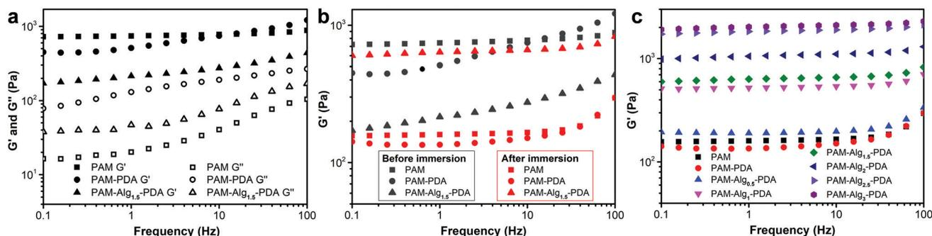
Fig. 5 The dynamic rheological behavior of various hydrogels. (a) The storage modulus ( $G'$ ) and loss modulus ( $G''$ ) of hydrogels before immersion in artificial seawater; (b) comparison of  $G'$  of hydrogels before and after immersion in seawater for 3 days; (c) the change in  $G'$  of hydrogels with the concentration of Alg–Na immersed in artificial seawater for 3 days.
