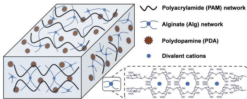
Scheme 1 Schematic structure of PAM-Alg-PDA hydrogel adhesive.
