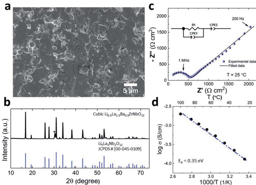
Fig. 1 (a) Cross-sectional SEM image of the LLZO SE. (b) XRD pattern for the synthesized LLZO compound confirming the formation of a cubic phase. \* Indicates the  $\text{BaZrO}_3$  impurity phase (c) Nyquist plot for LLZO SE at room temperature. (d) Arrhenius plot of the bulk conductivity of the LLZO SE over a temperature range of 25–100 °C.
