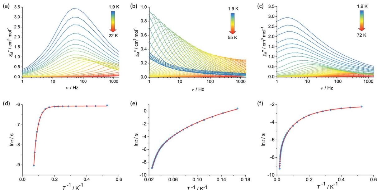
Fig. 2 Frequency dependence of the imaginary component of the AC susceptibility,  $\chi''$  versus  $\nu$ , in zero DC field for (a) 1, (b) 2 and (c)  $[3][\text{B}(\text{C}_6\text{F}_5)_4]$  at the temperatures indicated, and the temperature dependence of the relaxation time as  $\ln \tau$  versus  $T^{-1}$  for 1 (d), 2 (e) and (f)  $[3][\text{B}(\text{C}_6\text{F}_5)_4]$ .
