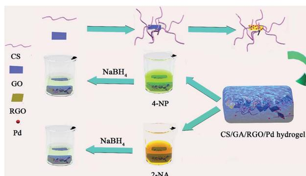
Fig. 1 Preparation and catalytic process of CS/GA/RGO/Pd hydrogel.
