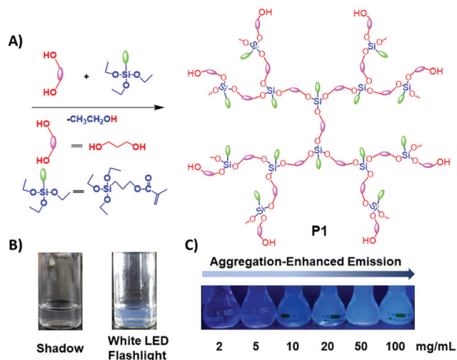
Fig. 1 (A) Synthetic route toward P1 ; (B) 15 mg mL -1 P1 ethanol solution under white LED flashlight or shadow; (C) P1 ethanol solution with different concentrations under 365 nm UV light.
