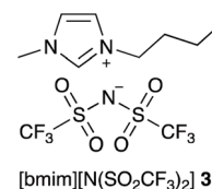
Fig. 1 The ionic liquid 1-butyl-3-methylimidazolium bis(trifluoromethanesulfonyl)imide ([bmim][N(SO 2 CF 3 ) 2 ], 3 ) used in this study. It should be noted that this anion might also be named as a secondary (sulfonyl)amide. 57 However, imide nomenclature is also reasonable 58 and serves to emphasise the two substituents, along with being consistent with previous work and what is used by the community in, for example, chemical catalogues.
