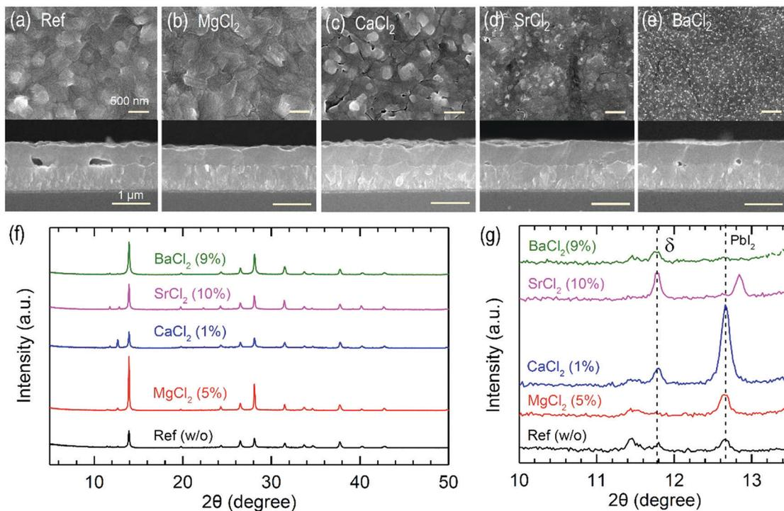
Fig. 3 (a–e) Top-view and cross-sectional scanning electron microscope (SEM) images and (f, g) X-ray diffraction patterns of FAPbI<sub>3</sub> films with and without (Ref) additives of MgCl<sub>2</sub>, CaCl<sub>2</sub>, SrCl<sub>2</sub> and BaCl<sub>2</sub>.
