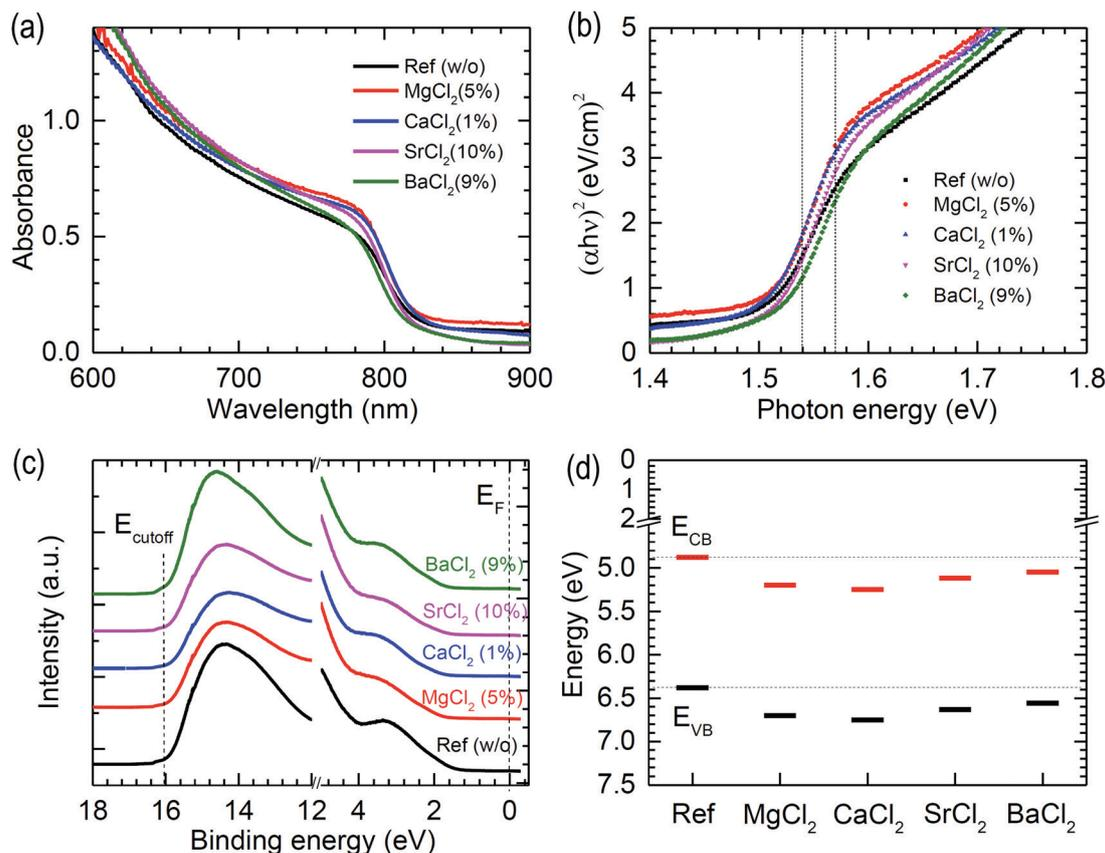
Fig. 6 (a) UV-vis spectra, (b) Tauc plot, (c) ultraviolet photoelectron spectroscopy (UPS) and (d) band (conduction band (CB) and valence band (VB)) positions for the FAPbI<sub>3</sub> films with and without additives. UPS spectra were measured with He I photon energy (21.2 eV).
