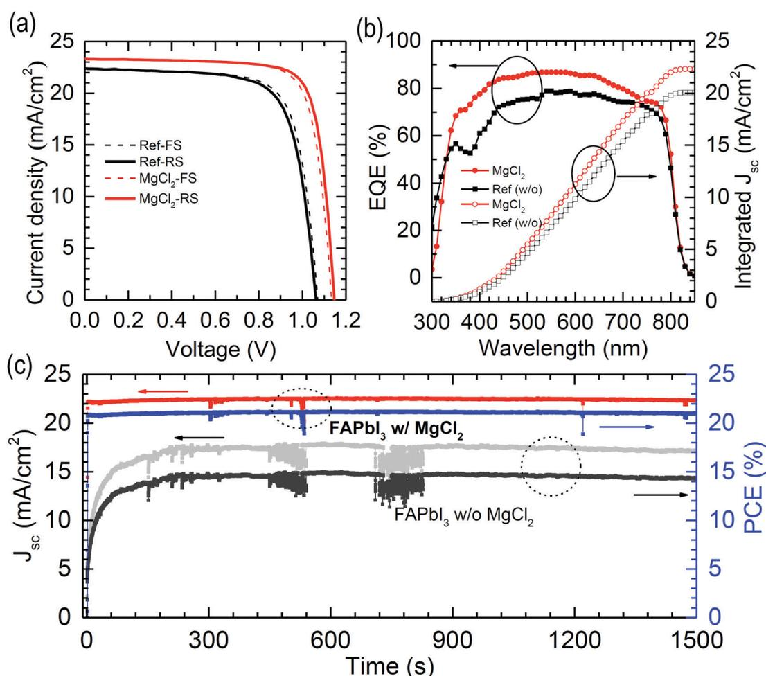
**Fig. 8** (a)  $J$ - $V$  curves and (b) external quantum efficiency (EQE) of PSCs employing FAPbI<sub>3</sub> with and without MgCl<sub>2</sub> additive. (c) Steady-state  $J_{sc}$  and PCE for the PSCs employing FAPbI<sub>3</sub> with and without the MgCl<sub>2</sub> additive, measured at the maximum power point (MPP) for 1500 s under continuous 1 sun illumination.
