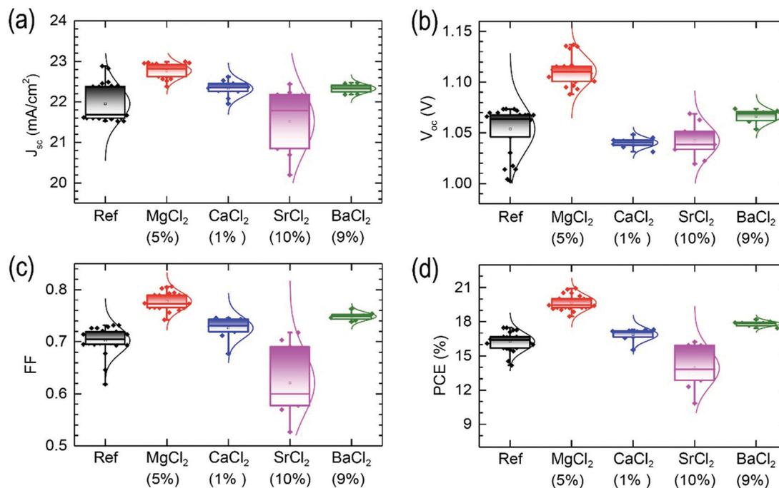
Fig. 2 Statistical photovoltaic parameters of (a)  $J_{sc}$ , (b)  $V_{oc}$ , (c) FF and (d) PCE measured at reverse scan for the BCl<sub>2</sub> additives (B = Mg, Ca, Sr and Ba). Values in parentheses are the optimal mol% of the additive with respect to FAPbI<sub>3</sub>.
