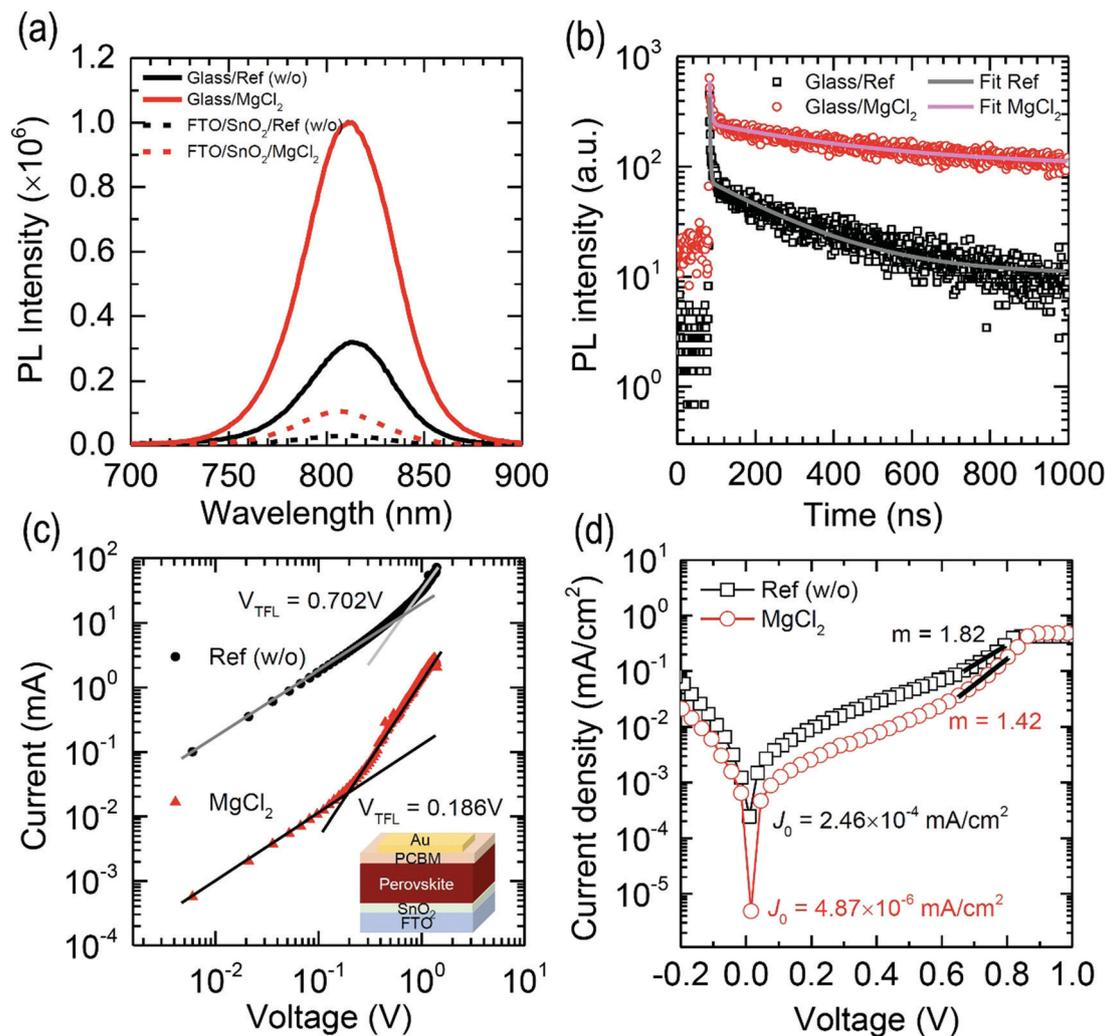
Fig. 7 (a) Steady-state photoluminescence (PL) of the FAPbI<sub>3</sub> film with and without MgCl<sub>2</sub> deposited on a glass substrate and SnO<sub>2</sub>-coated FTO substrate. (b) Time-resolved PL (TRPL) for the FAPbI<sub>3</sub> film with and without MgCl<sub>2</sub> on a glass substrate. Dark current density ( $J$ )–voltage ( $V$ ) curves for (c) the FTO/SnO<sub>2</sub>/FAPbI<sub>3</sub> (with or without MgCl<sub>2</sub>)/PCBM/Au electron-only device and (d) the full solar cell device.
