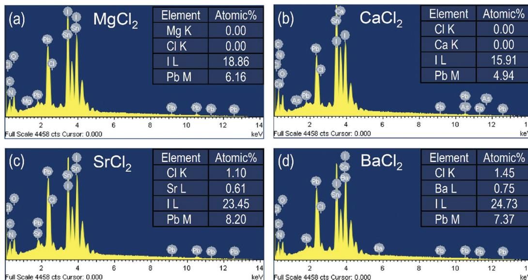
Fig. 4 Energy dispersive X-ray spectroscopy (EDS) of FAPbI<sub>3</sub> films with additive of (a) MgCl<sub>2</sub> (5%), (b) CaCl<sub>2</sub> (1%), (c) SrCl<sub>2</sub> (10%) and (d) BaCl<sub>2</sub> (9%).
