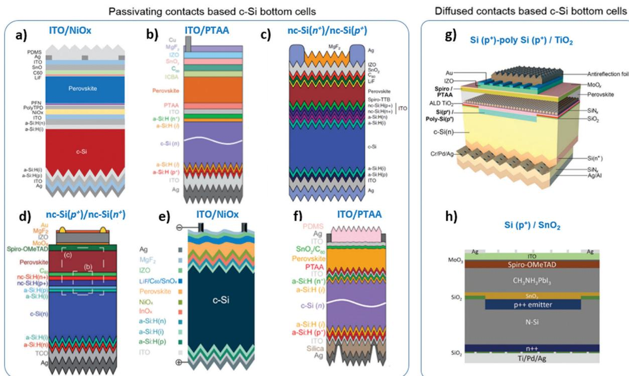
Fig. 4 Representative examples of the successful RJs used in literature for passivating contacts and diffused-junction contacts based c-Si bottom cells (References: a,<sup>55</sup> b,<sup>56</sup> c,<sup>49</sup> d,<sup>33</sup> e,<sup>57</sup> f,<sup>58</sup> g,<sup>59</sup> h<sup>60</sup> reprint with permissions).
