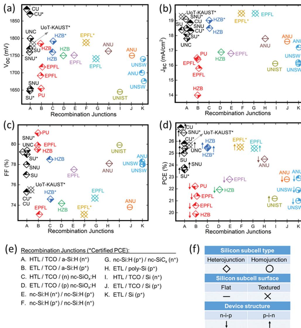
Fig. 5 (a)  $V_{oc}$ , (b)  $J_{sc}$ , (c) FF and (d) PCE values of the reported silicon/perovskite monolithic tandem solar cells with different RJs. Descriptions for the RJs (e) and tandem device indicators (f). The asterisks represent independently certified values.
