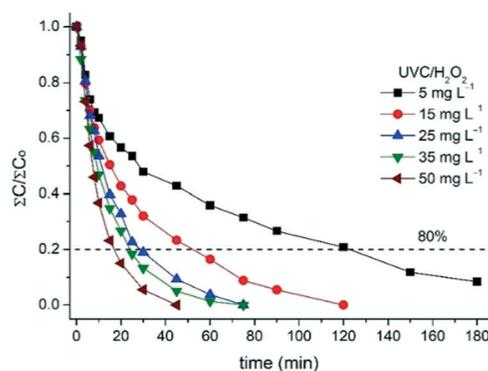
**Fig. 4** Effect of H<sub>2</sub>O<sub>2</sub> concentration on the total MC degradation by UVC/H<sub>2</sub>O<sub>2</sub> as a function of treatment time in SMWW secondary effluent. Dashed line refers to 80% removal of total MCs ( $\sum C_t/\sum C_0$ ).
