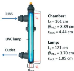
Fig. 1 UVC photoreactor scheme and main characteristics.
