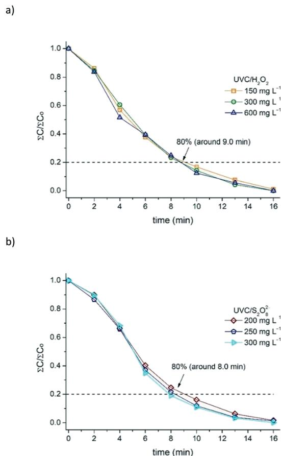
Fig. 7 Effect of high concentration of oxidant on the total MC degradation under UVC irradiation as a function of treatment time in SMWW secondary effluent: (a)  $\text{H}_2\text{O}_2$  and (b)  $\text{S}_2\text{O}_8^{2-}$ . Dashed lines refer to 80% removal of total MCs ( $\Sigma C_i / \Sigma C_0$ ).
