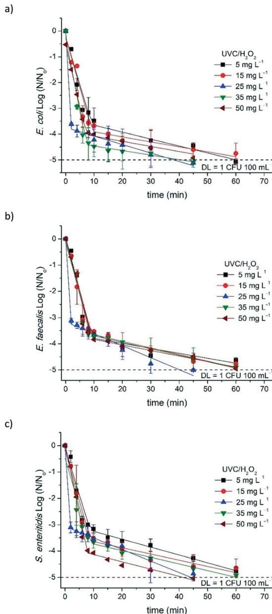
Fig. 3 Effect of H<sub>2</sub>O<sub>2</sub> concentration on the *E. coli* (a), *E. faecalis* (b), and *S. enteritidis* (c) inactivation by UVC/H<sub>2</sub>O<sub>2</sub> as a function of treatment time in SMWW secondary effluent. Dashed lines refer to detection limit (DL = 1 CFU per 100 mL<sup>-1</sup>).
