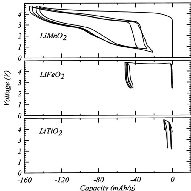
Fig. 13 Electrochemical profiles from cathodes prepared from  $\text{LiMnO}_2$ ,  $\text{LiFeO}_2$  and  $\text{LiTiO}_2$  milled for 48 h. Reprinted from M. N. Obrovac, O. Mao, J. R. Dahn, Structure and electrochemistry of  $\text{LiMO}_2$  ( $M = \text{Ti, Mn, Fe, Co, Ni}$ ) prepared by mechanochemical synthesis,<sup>8</sup> *Solid State Ionics*, vol. 112, pp. 9–19, copyright 1998, with permission from Elsevier.
