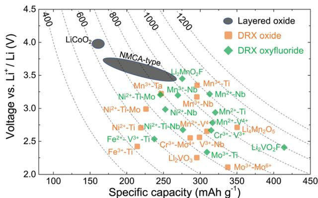
Fig. 2 Average discharge potential (V vs.  $\text{Li}^+/\text{Li}$ ) and gravimetric capacity ( $\text{mAh g}^{-1}$ ) of selected layered and DRX cathodes. Contour lines represent the gravimetric energy density ( $\text{Wh kg}^{-1}$ ). NMCA = NMC (Li–Ni–Mn–Co–O<sub>2</sub>) and NCA (Li–Ni–Co–Al–O<sub>2</sub>).
