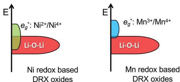
Fig. 14 Qualitative diagrams of transition metal and oxygen electronic states in Ni<sup>2+</sup>/Ni<sup>4+</sup> redox-based and Mn<sup>3+</sup>/Mn<sup>4+</sup> redox-based DRXs.
