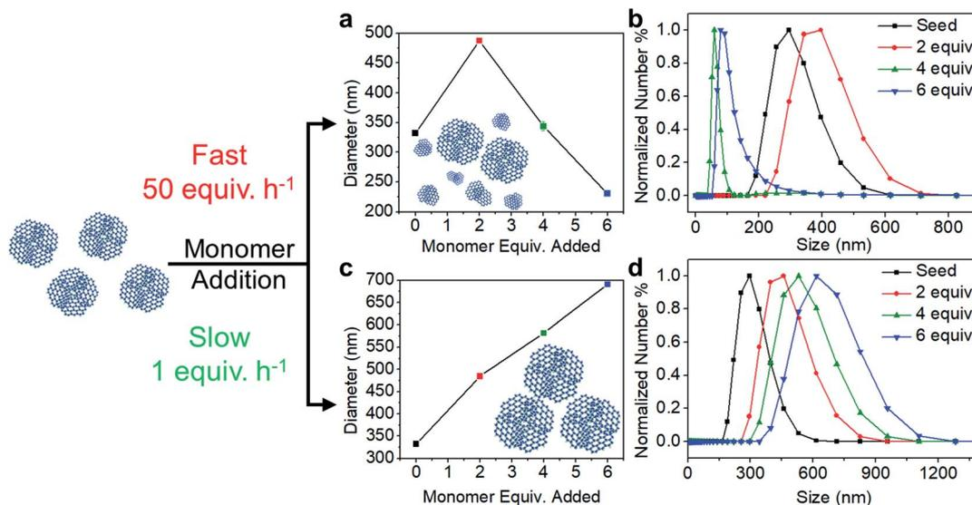
Fig. 3 Trend in the average size of particles with monomer addition at a fast rate of 50 equiv. h<sup>-1</sup> and at a slow rate of 1 equiv. h<sup>-1</sup>. (a, c) Average size of particles with additional equivalents of monomers (b, d) corresponding number percent distribution.
