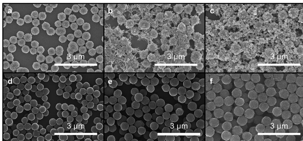
Fig. 4 SEM images of colloidal suspension at 50 equiv. h<sup>-1</sup> (a–c) and 1 equiv. h<sup>-1</sup> (d–f) of monomer addition. Aliquots were drop-casted after (a, d) 2 equivalents, (b, e) 4 equivalents, and (c, f) 6 equivalents of monomers were added.
