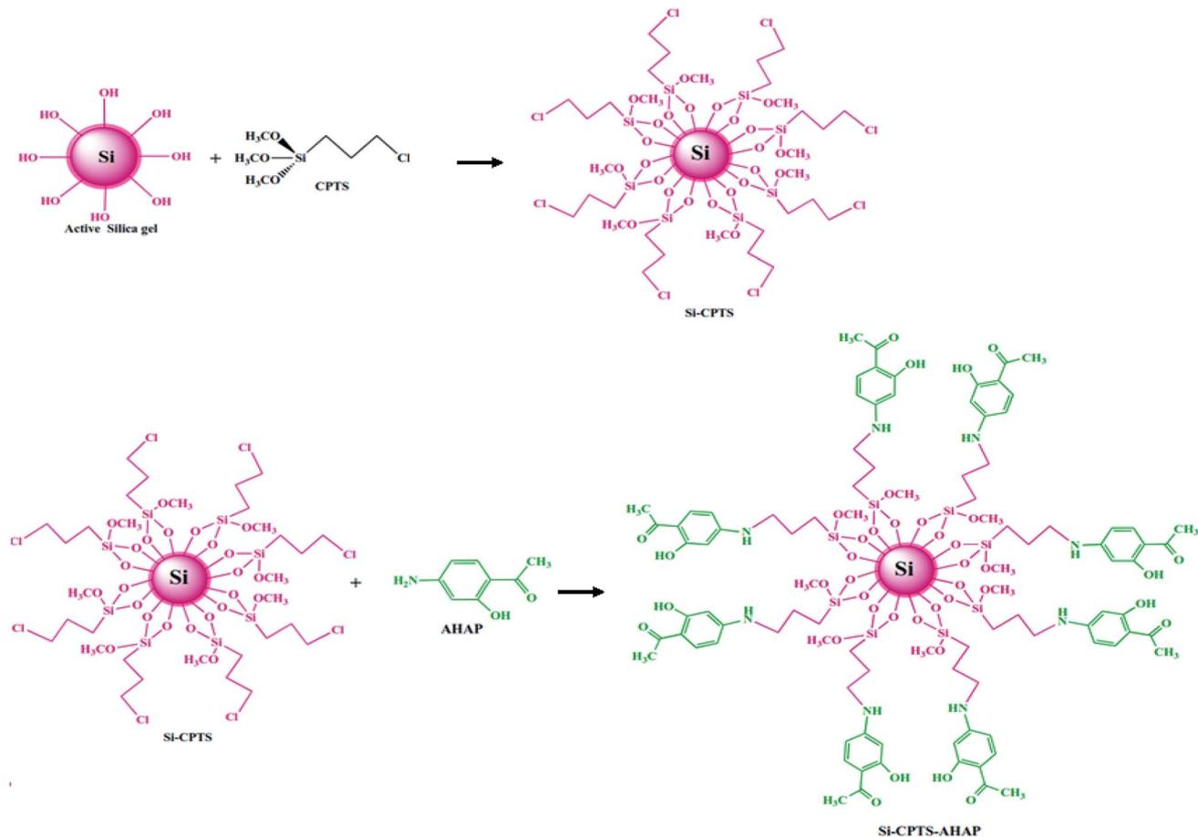
Fig. 1 Possible structure of the synthesized Si-CPTS-AHAP adsorbent.
