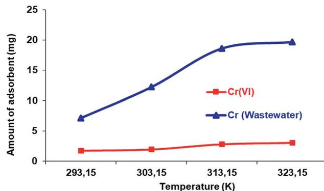
Fig. 6 The effect of temperature on the adsorption of Cr(vi) from aqueous solution and wastewater.
