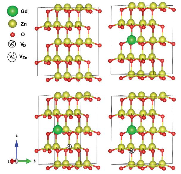
Crystal structures of pristine, Gd-doped ZnO and Gd-complex defects ZnO
