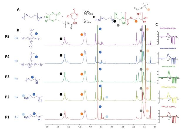
Fig. 2 (A) general reaction scheme for the PEG-initiated ROP, (B) <sup>1</sup>H NMR spectra of the five copolymers (with random distribution of ester and carbonate units) and (C) GPC traces of the polymers.
