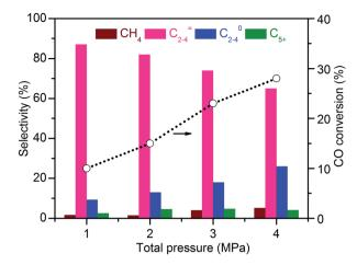
Fig. 9 Effect of total pressure of syngas on catalytic behaviours of Zn–ZrO<sub>2</sub>/SSZ-13–45H catalyst. Reaction conditions: catalyst, 0.60 g;  $H_2/CO = 2/1$ ; T = 673 K; F = 30 mL min<sup>-1</sup>; time on stream, 10 h.
