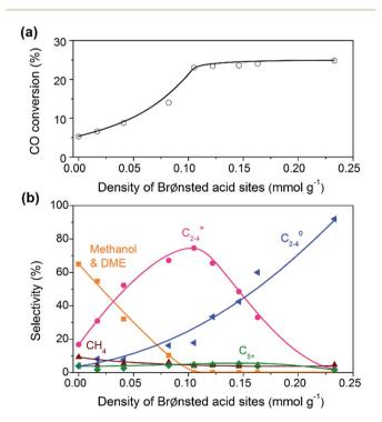
Fig. 5 Effect of density of Brønsted acid sites on catalytic behaviours of the bifunctional Zn–ZrO<sub>2</sub>/SSZ-13 catalyst. (a) CO conversion. (b) Product selectivity. The selectivity of CO<sub>2</sub> did not change with the density of Brønsted acid sites and was in the range of 41–45%. Reaction conditions: catalyst, 0.60 g;  $H_2/CO = 2$ ; P = 3 MPa; T = 673 K; F = 30 mL min<sup>-1</sup>; time on stream, 10 h.
