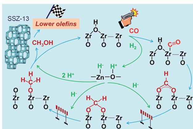
Fig. 13 A possible reaction mechanism for the conversion of syngas into lower olefins over Zn-ZrO<sub>2</sub>/SSZ-13 catalyst.
