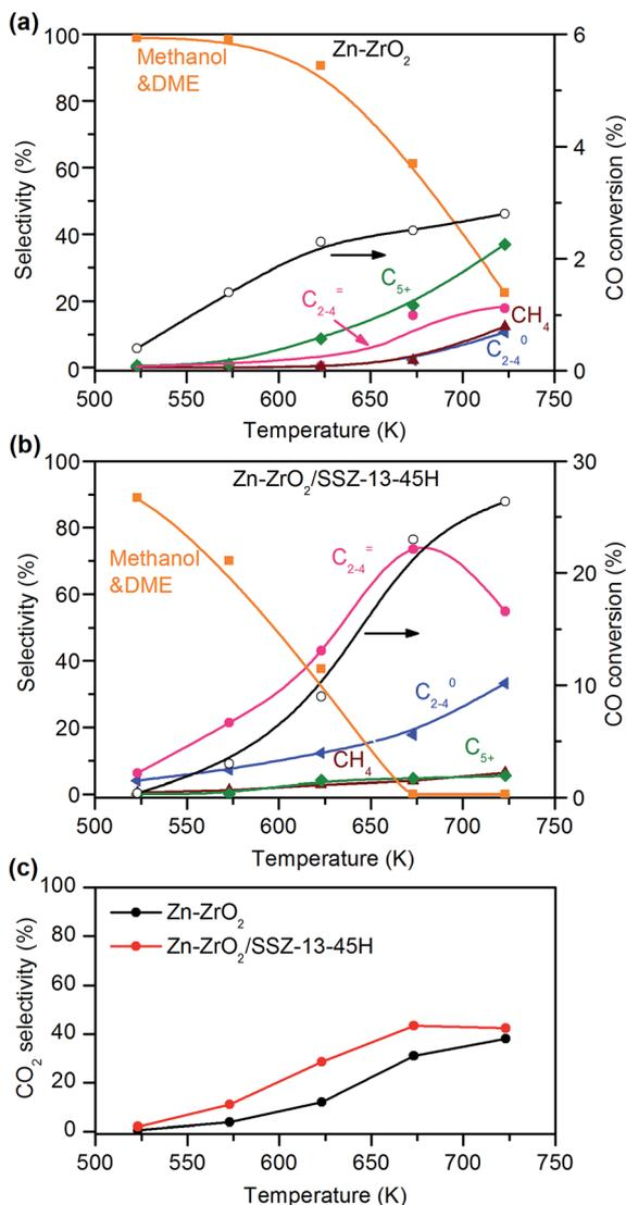
Fig. 2 Catalytic behaviours of Zn-ZrO<sub>2</sub> and Zn-ZrO<sub>2</sub>/SSZ-13-45H catalysts for the conversion of syngas at different temperatures. (a) Zn-ZrO<sub>2</sub> (Zn/Zr = 1 : 16). (b) Zn-ZrO<sub>2</sub>/SSZ-13-45H. (c) CO<sub>2</sub> selectivity. Reaction conditions:  $W(\text{Zn-ZrO}_2) = 0.20 \text{ g}$ ;  $W(\text{Zn-ZrO}_2/\text{SSZ-13-45H}) = 0.60 \text{ g}$ ;  $\text{H}_2/\text{CO} = 2$ ;  $P = 3 \text{ MPa}$ ;  $F = 30 \text{ mL min}^{-1}$ ; time on stream, 10 h.
