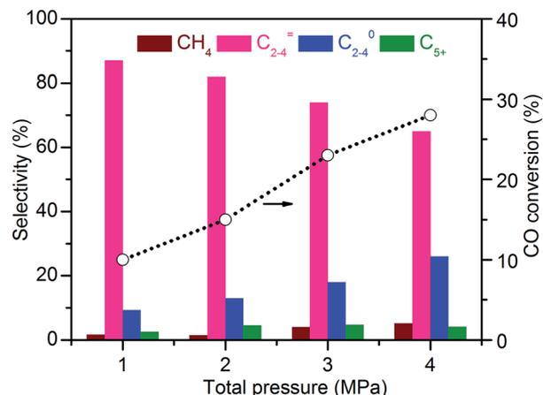
Fig. 9 Effect of total pressure of syngas on catalytic behaviours of Zn-ZrO<sub>2</sub>/SSZ-13-45H catalyst. Reaction conditions: catalyst, 0.60 g;  $\text{H}_2/\text{CO} = 2/1$ ;  $T = 673$  K;  $F = 30$  mL min<sup>-1</sup>; time on stream, 10 h.
