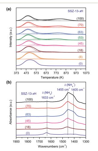
Fig. 4 Characterization of acidity of SSZ-13 with different  $H^+$ -exchanging degrees. (a)  $NH_3$ -TPD profiles. (b)  $NH_3$ -adsorbed FT-IR spectra. The number in the parentheses after each sample denotes the  $H^+$ -exchanging degree.
