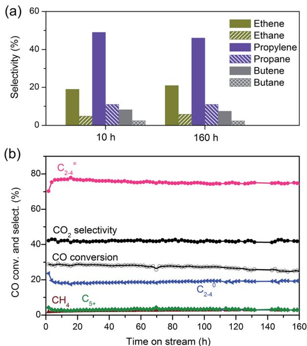
Fig. 7 (a) Selectivities of C<sub>2</sub>, C<sub>3</sub> and C<sub>4</sub> olefins and paraffins over Zn-ZrO<sub>2</sub> (4.8 nm)/nano-SSZ-13. (b) Stability of Zn-ZrO<sub>2</sub> (4.8 nm)/nano-SSZ-13 catalyst. Reaction conditions: catalyst, 0.60 g; H<sub>2</sub>/CO = 2; P = 3 MPa; T = 673 K; F = 30 mL min<sup>-1</sup>.
