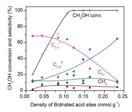
Fig. 11 Effect of density of Brønsted acid sites for the conversion of methanol over SSZ-13 zeolites. Reaction conditions: catalyst, 0.4 g;  $F(H_2) = 30 \text{ mL min}^{-1}$ ;  $F(\text{liquid CH}_3\text{OH}) = 0.01 \text{ mL min}^{-1}$ ; P = 2 MPa; T =673 K; time on stream, 3 h.
