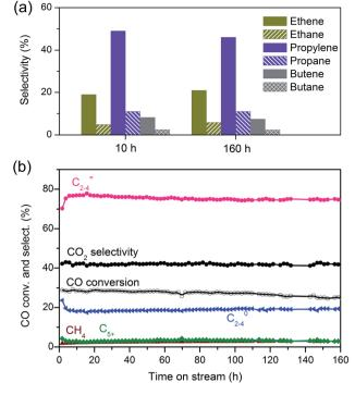
Fig. 7 (a) Selectivities of  $C_2$ ,  $C_3$  and  $C_4$  olefins and paraffins over Zn–ZrO<sub>2</sub> (4.8 nm)/nano-SSZ-13. (b) Stability of Zn–ZrO<sub>2</sub> (4.8 nm)/nano-SSZ-13 catalyst. Reaction conditions: catalyst, 0.60 g; H<sub>2</sub>/CO = 2; P = 3 MPa; T = 673 K; F = 30 mL min<sup>-1</sup>.
