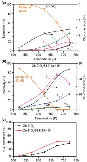
Fig. 2 Catalytic behaviours of Zn–ZrO $_2$  and Zn–ZrO $_2$ /SSZ-13–45H catalysts for the conversion of syngas at different temperatures. (a) Zn–ZrO $_2$  (Zn/Zr = 1 : 16). (b) Zn–ZrO $_2$ /SSZ-13–45H. (c) CO $_2$  selectivity. Reaction conditions: W(Zn–ZrO $_2$ ) = 0.20 g; W(Zn–ZrO $_2$ /SSZ-13–45H) = 0.60 g; H $_2$ /CO = 2; P = 3 MPa; F = 30 mL min $^{-1}$ ; time on stream, 10 h.
