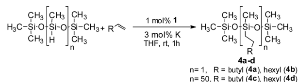
Scheme 3 The hydrosilylation of olefins by siloxanes.
