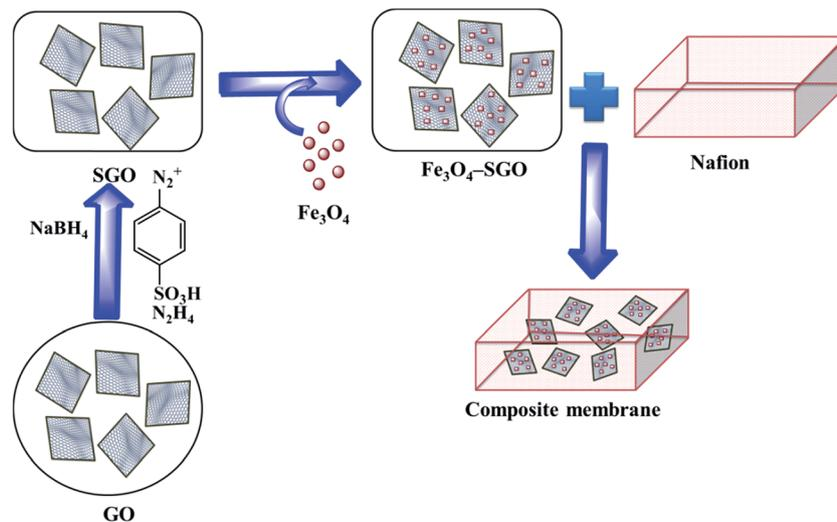
Scheme 1 Preparation process of Nafion/Fe<sub>3</sub>O<sub>4</sub>-SGO composite membrane.
