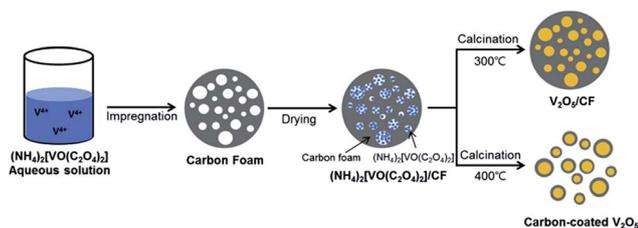
Fig. 12 Schematic of the preparation of carbon-fabricated V<sub>2</sub>O<sub>5</sub> samples (CF300 and CF400).<sup>117</sup>
