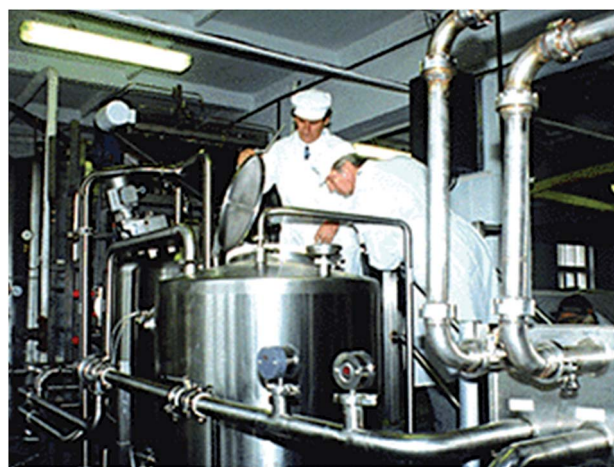
Fig. 5 The MAG*SEP SM milk decontamination system at Ovruch, Ukraine 1997. 1
