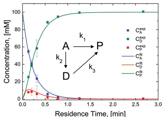
**Fig. 4** Lumped kinetic mechanism determination. Experimental concentration profiles (datapoints), are deconvoluted from the reactor effluent and plotted *versus* mean residence time for the starting material (**A**), the intermediate (**D**) and the product (**P**), with total mass closure of >93%. Model fits (solid lines) correspond with lumped kinetic rate constants  $k_1 = 0.31 \text{ min}^{-1}$ ,  $k_2 = 2.25 \text{ min}^{-1}$ ,  $k_3 = 11.07 \text{ min}^{-1}$ .
