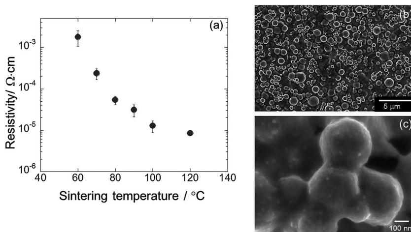
Fig. 29 (a) Change in electrical resistivity of Cu films as a function of sintering temperature. (b, c) SEM images of the sintered Cu films prepared after sintering at 80  $^{\circ}\text{C}$ . [Reprinted with permission from ref. 269 Copyright  $\copyright$  American Chemical Society.]
