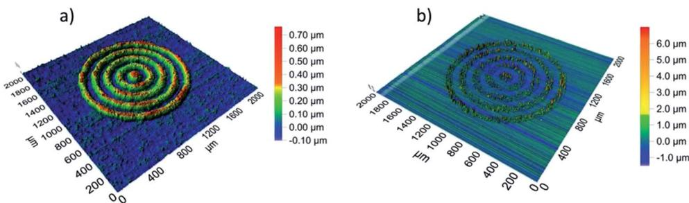
**Fig. 17** A comparison of the topography of (a) thermally and (b) photonically sintered silver molecular ink traces analyzed from optical profilometry. [Reprinted with permission from ref. 231 Copyright © American Chemical Society.]
