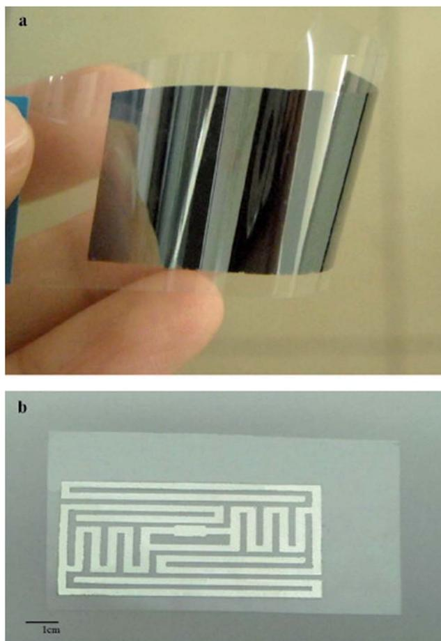
Fig. 25 (a) Photograph of inkjet printed silver patterns on PET substrate showing the metallic luster. (b) Inkjet printed silver ink based RFID antenna. [Reprinted with permission from ref. 120 Copyright © Elsevier.]
