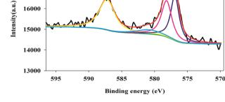
Fig. 5 XPS analysis of the TW/Fe<sub>3</sub>O<sub>4</sub> composite and absorbed Cr on the TW/Fe<sub>3</sub>O<sub>4</sub> composite (a) TW/Fe<sub>3</sub>O<sub>4</sub> composite (b) Cr laden on the TW/Fe<sub>3</sub>O<sub>4</sub> composite (c) speciation analysis of Cr.
