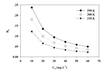
Fig. 10 The variation of  $R_{\rm L}$  under different initial concentrations and temperatures.
