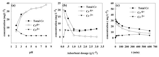
Fig. 12 Concentration of total Cr. Cr(yı), Cr(yı), under different parameters (a) pH (b) adsorbent mass (c) contact time.
