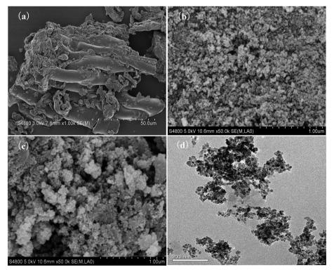
Fig. 1 SEM photo (a) tea waste; (b) Fe<sub>3</sub>O<sub>4</sub>; (c) TW/Fe<sub>3</sub>O<sub>4</sub> composite and (d) TEM of TW/Fe<sub>3</sub>O<sub>4</sub> composite.
