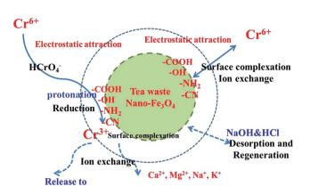
Fig. 14 Proposed mechanism of Cr(vi) removal by the TW/Fe<sub>3</sub>O<sub>4</sub> composite.
