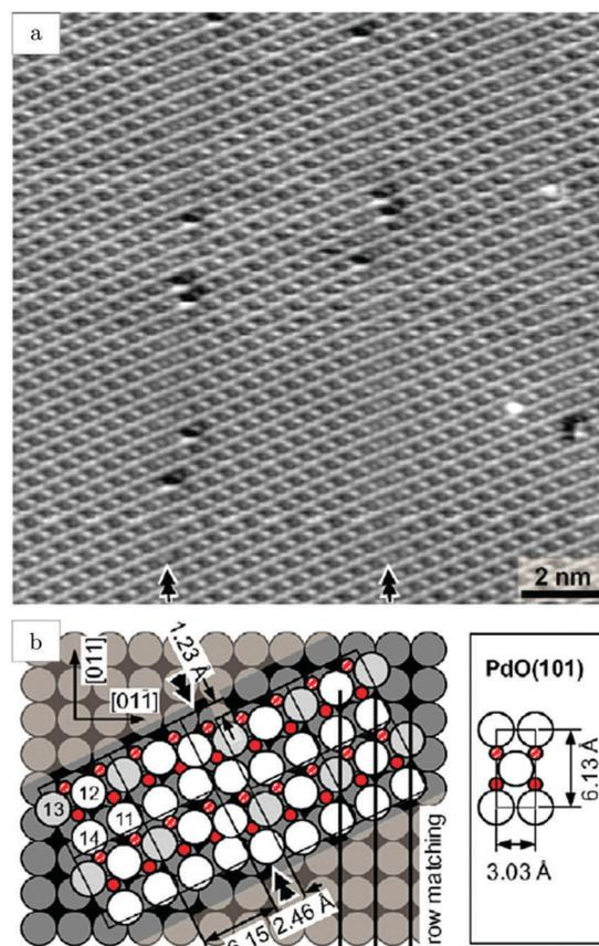
Fig. 12 STM image (a) of the ( $\sqrt{5} \times \sqrt{5}$ )R27° surface oxide on Pd(100) in UHV. Arrows indicate domain boundaries. Ball model for this oxide (b). Reproduced from ref. 121 with permission from Elsevier, copyright 2007.
