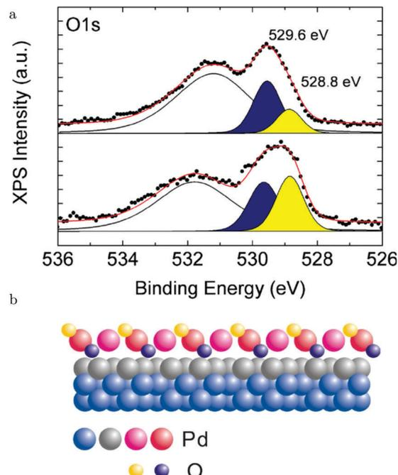
Fig. 18 XPS measurements (a) on Pd(100) under CO oxidation conditions for the O 1s region at  $\sim 483$  K (lower panel) and 643 K (upper panel). The broad peak originated from Pd  $3p_{3/2}$  photoelectrons. (b) Model of the  $\sqrt{5}$  surface oxide with the two different types of O atoms (reactive, 528.8 eV, and inactive, 529.6 eV). Reproduced from ref. 129 with permission from the American Chemical Society, copyright 2012.
