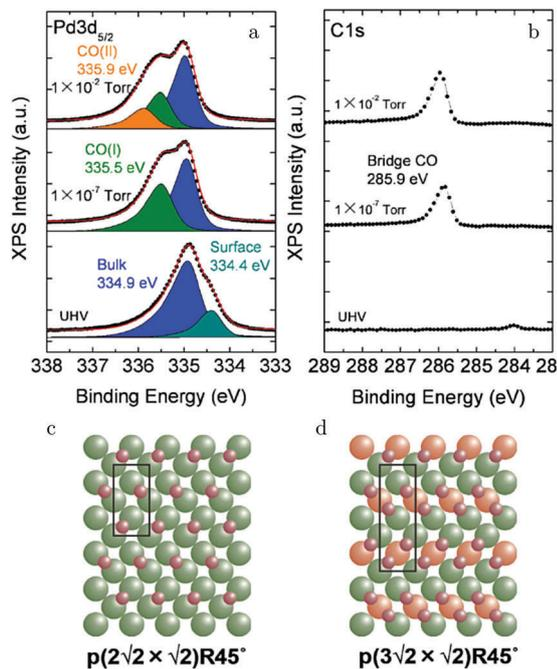
Fig. 17 XPS measurements on Pd(100) [Pd  $3d_{5/2}$  (a) and C 1s (b)] for increasing  $p_{\text{CO}}$  at RT. Models of the CO(ads) layers for 0.5 ML (c) and 0.67 ML (d). Reproduced from ref. 129 with permission from the American Chemical Society, copyright 2012.
