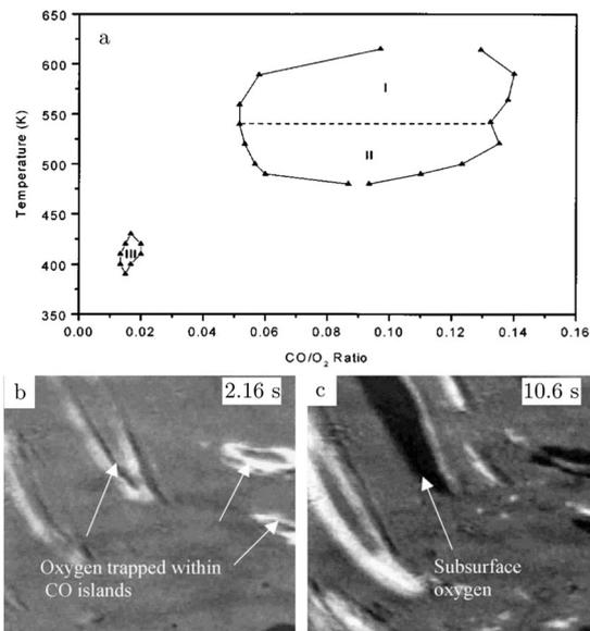
**Fig. 10** Diagram (a) of conditions probed in the intermediate pressure regime of several Pa, for which nonlinear dynamics was observed. EMSI images (b and c) showing the complex pattern of adsorbate islands on the surface and the formation of chemisorbed O ( $1 \times 1.25 \text{ mm}^2$ ,  $\chi = 0.13$ , 8 Pa, and 523 K). Reproduced from ref. 92 with permission from Wiley, copyright 2001 (a) and from ref. 93 with permission from Elsevier, copyright 2005 (b and c).
