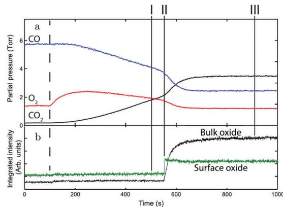
**Fig. 14** (a) Gas-phase information, while decreasing the CO pressure at 525 K. (b) Intensity of diffraction peaks of the surface oxide (green) and the bulk oxide (black) on Pd(100), recorded with high-energy SXRD. Reproduced from ref. 110 with permission from Science, copyright 2014.
