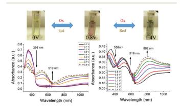
Fig. 4 Spectroelectrochemistry of 3,6-Cbz-EDOT films on an ITO electrode measured in CH<sub>3</sub>CN with 0.1 M (nC<sub>4</sub>H<sub>9</sub>)<sub>4</sub>NPF<sub>6</sub>.
