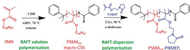
**Scheme 1** Synthesis of a PSMA<sub>14</sub> macro-CTA by RAFT solution polymerisation of SMA followed by the preparation of PSMA<sub>14</sub>-PNMEP<sub>x</sub> nano-objects *via* RAFT dispersion polymerisation of NMEP in *n*-dodecane at 90 °C.
