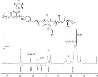
Fig. 1  $\,^{1}$ H NMR spectrum (400 MHz, CDCl $_{3}$ ) of PLLA-b-PMAC-b-PTHPA triblock copolymer, 4.
