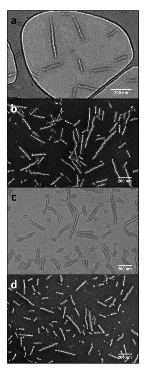
**Fig. 3** TEM images showing the PLLA-*b*-PMAC-*b*-PAA cylindrical micelles before (a and b) and after functionalization with benzyl mercaptan (c and d). a and c, on graphene oxide grid;<sup>49</sup> b and d, with negative staining using phosphotungstic acid (PTA). Scale bar = 200 nm.
